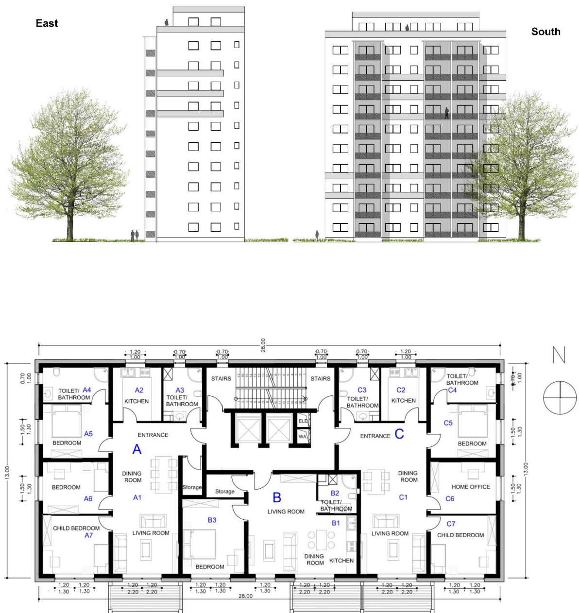
Figure 2: East and south view and floor plan of the ‘passive house high-rise’ building model
