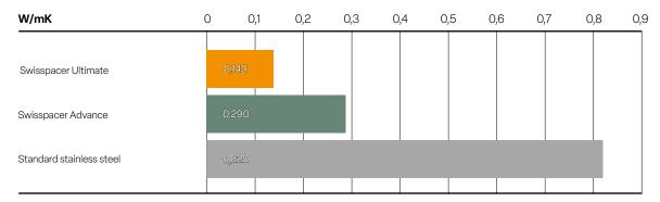
Equivalent thermal conductivity in W/mK according to EN 12664:2001-01 and ift guideline WA17/1
